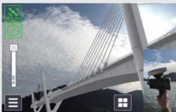
Review of construction progress based on the technology of GNSS-AR
